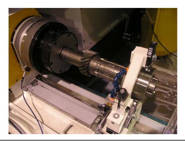
Powerhold's new Compensating Collet Chuck gives you the ability to automate an operation that historically has required springs and drive-dogs. The chuck has a centerpoint for location and a collet to grip the part OD. The drawbar-actuated collet compensates to ensure the part is not pushed off location. Couple this chuck with a steady rest and now you can ID grind long parts.
